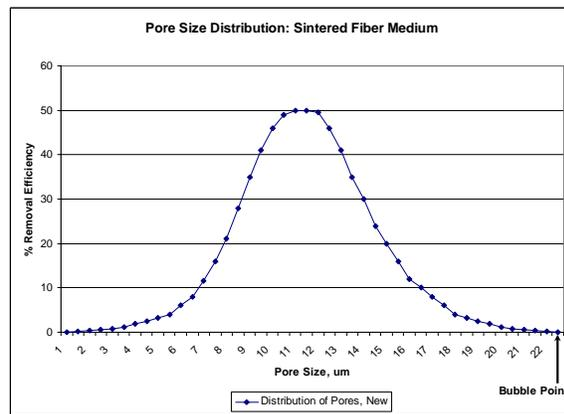
Figure 2B: Sintered Fiber Medium Pore Size Distribution and Bubble Point
