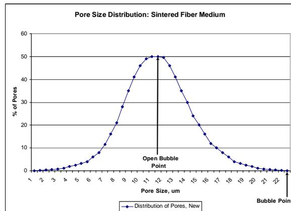
Figure 3B: Sintered Fiber Medium Pore
