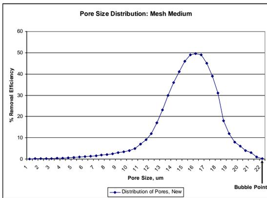
Figure 2A: Mesh Medium Pore Size Distribution and Bubble Point
